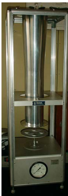
Figura 5. Torre Potter ST-4
