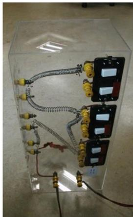
Figura 3.6. Carga resistiva variable.
