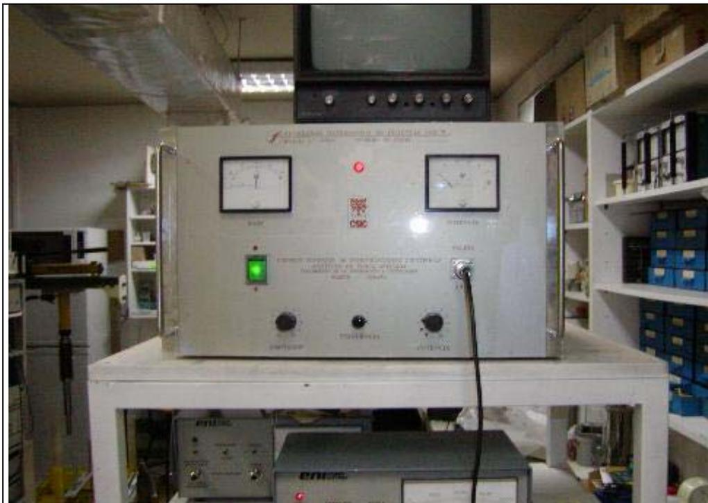
Figura 10. ENI Power Meter (Potentiometer). Model EMB 2K 250.
