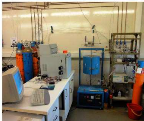
Figure 1. Schematic representation and picture of the experimental steam reforming unit: (1) feeding gases; (2) mass-flow controllers; (3) feeding ethanol-water mixture; (4) pump for liquids; (5) mixing valve; (6) reforming reactor; (7) heating furnace; (8) catalyst layer; (9) sorbent layer; (10) back pressure valve; (11) condenser; (12) moisture trap; (13) gas-chromatograph.
