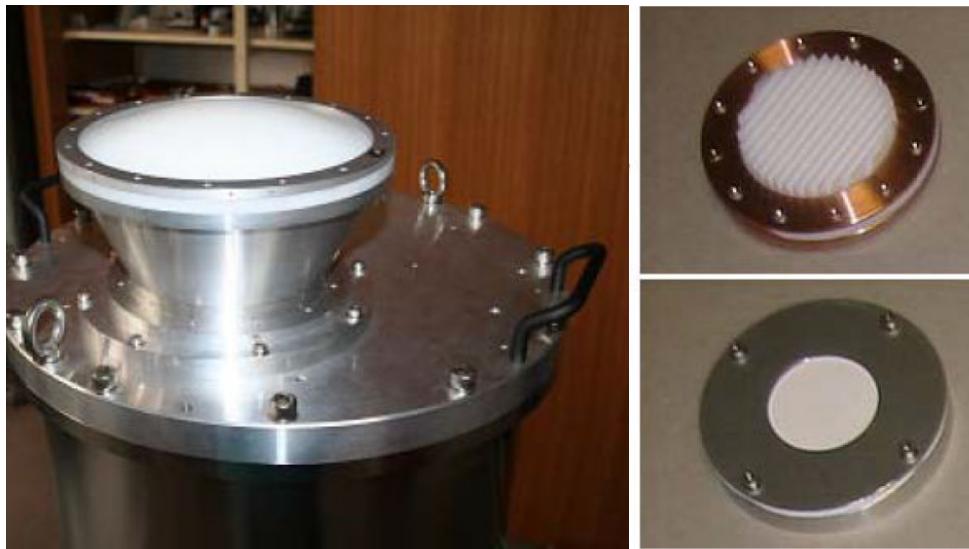
Figure 5.6: Left, prototyped lens installed on the test cryostat. Right, IR filters, Top is the 80 K filter and bottom is the 15 K filter.
