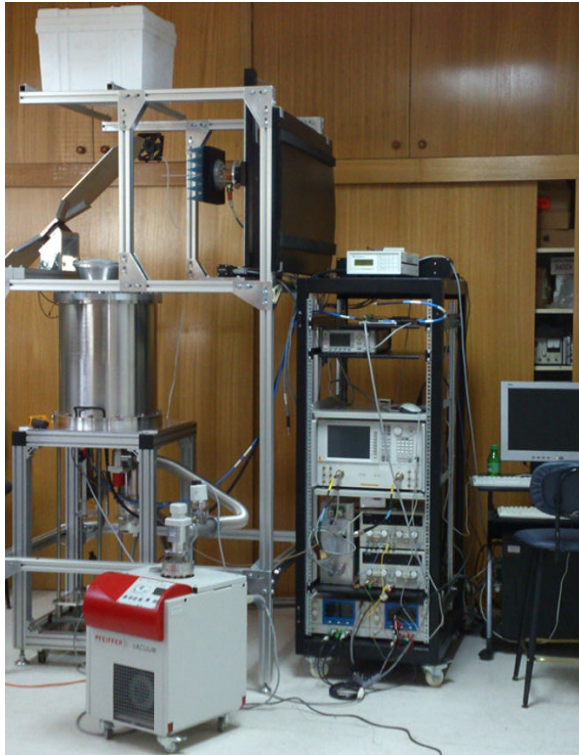
Figure 5.20: Test setup for receiver characterization. An ALMA compatible cryostat, developed by NAOJ is used to house the receiver.
