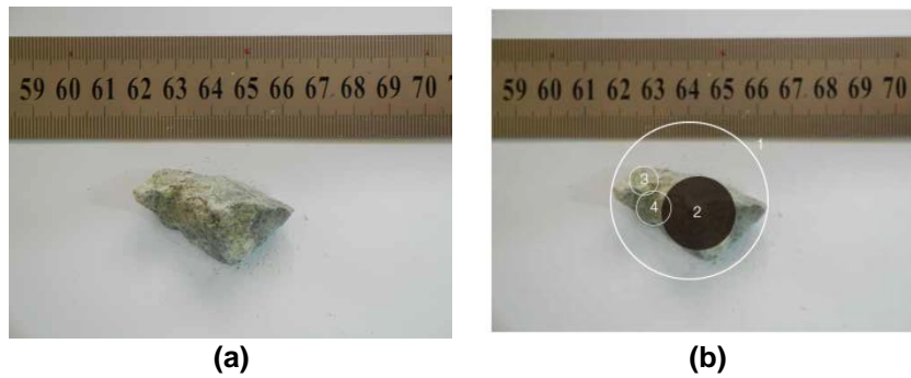
Figura 38: Mineral fragmento (# DSCN1414) (a) Fragmento d_{63,2} (b) Fragmento d_{63,2} evaluado
