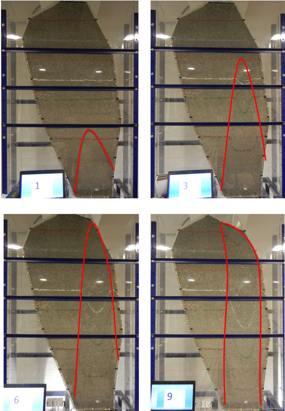
Figure 6.4. (Left Up) 1 kton from each drawpoint. (Right Up) 4 kton from each drawpoint. (Left Down) 10 kton from each drawpoint. (Right Up) 15 kton from each drawpoint.
