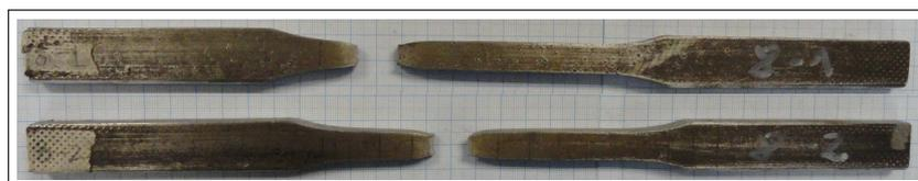
Figura 6.8: Probetas planas de 8 [mm]
