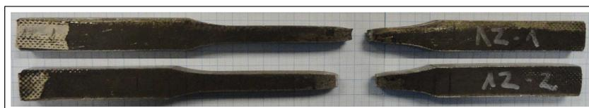
Figura 6.12: Probetas planas de 12 [mm]
