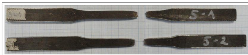
Figura 6.4: Probetas planas de 5 [mm]
