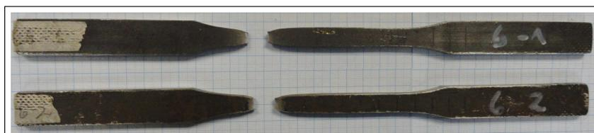
Figura 6.6: Probetas planas de 6 [mm]
