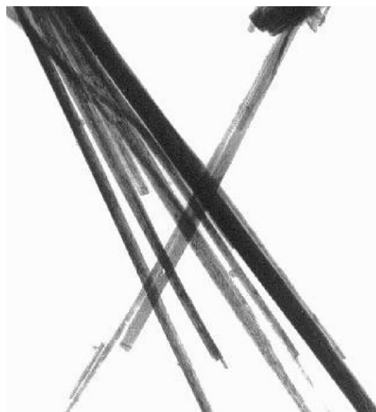
Fig. 6. TEM image of the product obtained at 150 °C during 72 h in absence of amine.
