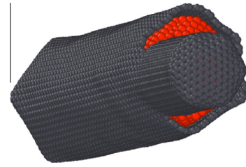
Fig. 11. Illustration of how two open ended misaligned different diameter iron filled CNTs stick together at the end (stage h of Fig. 10) of the soldering process shown in detail in Fig. 10.
