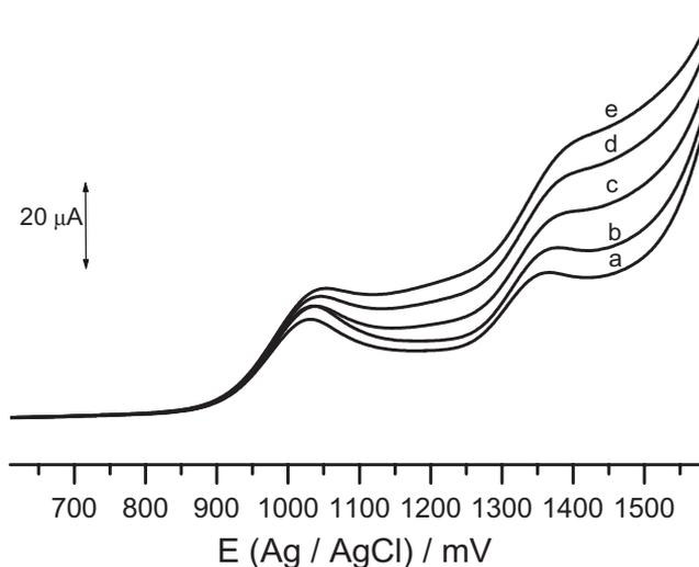
**Figure 3.** Typical hydrodynamic voltammograms on glassy carbon rotating disk electrode of 1 mM 4-(3-indolyl)-DHP in DMSO + 0.1 M TBAPF6 at different rotation rates: a = 100 rpm, b = 300 rpm, c = 500 rpm, d = 600 rpm, and e = 800 rpm.
