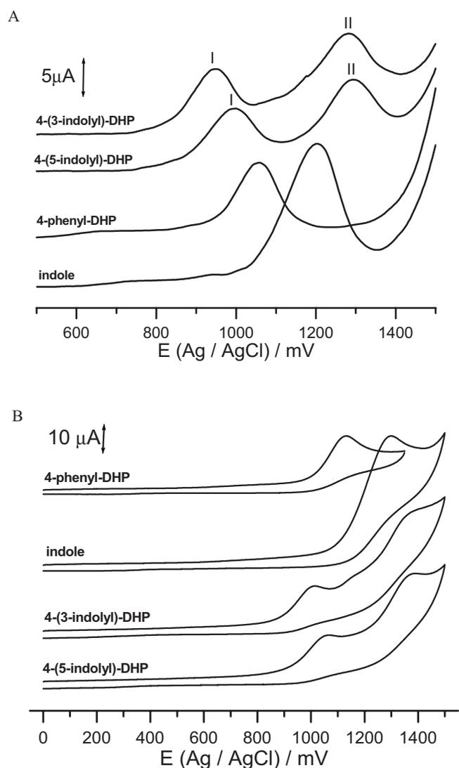
**Figure 2.** DPV (A) and cyclic voltammograms at 0.1 V/s (B) of 1 mM solutions of 4-(3-indolyl)-DHP, 4-(5-indolyl)-DHP, 4-phenyl-DHP, and indole in dimethylsulfoxide + 0.1 M TBAPF6.
