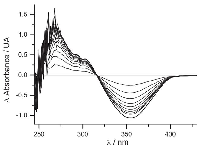
**Figure 4.** UV/vis differential spectra for the time course of CPE at +1100 mV for a 100  $\mu$ M 4-(3-indolyl)-DHP solution followed during 90 min.
