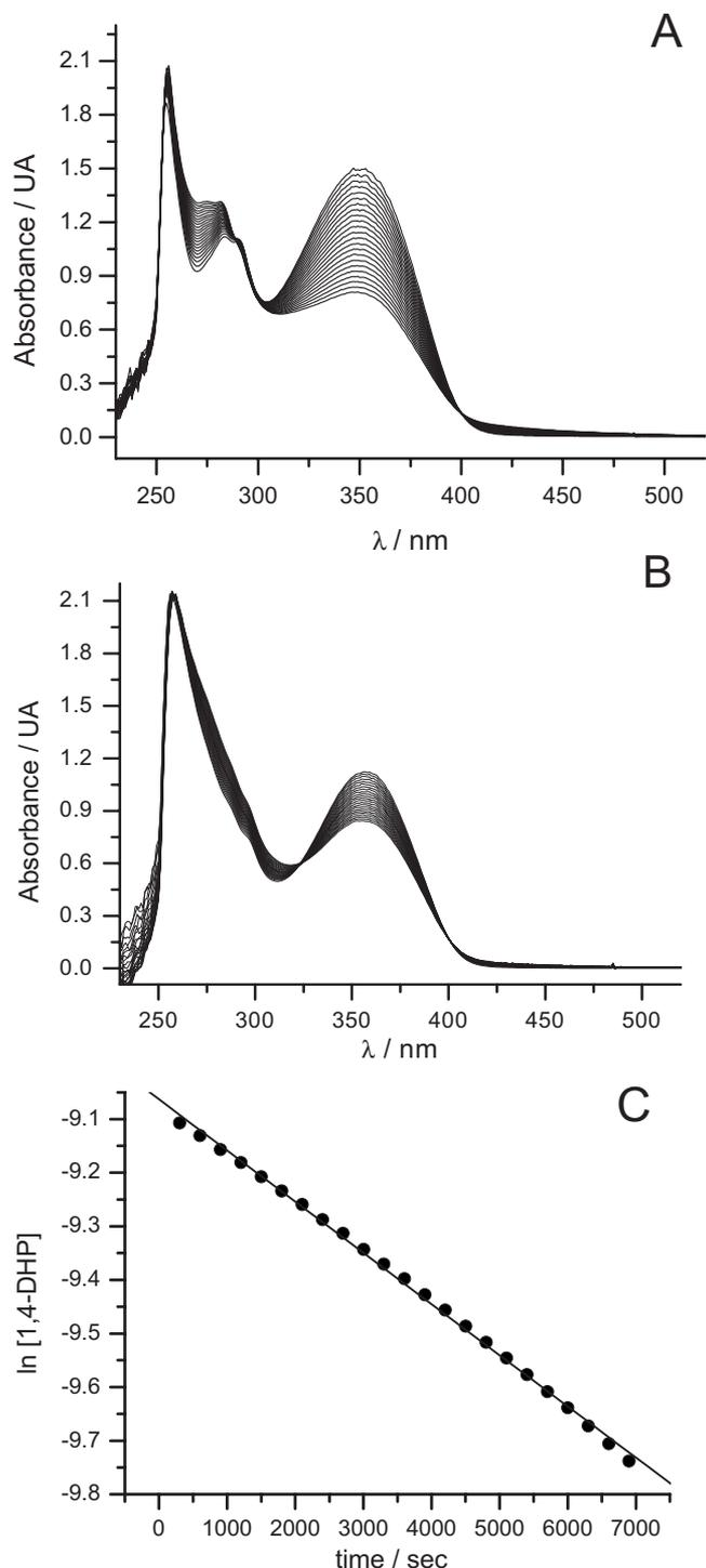
**Figure 7.** (A): UV/Vis spectra for the reaction between 4-(3-indolyl)-DHP and ABAP-derived alkylperoxyl radicals. (B): UV/vis spectra for the reaction between 4-phenyl-DHP and ABAP-derived alkylperoxyl radicals followed during 120 min. Reaction medium: 0.04 M Britton–Robinson buffer/DMF (70/30), pH 7.4 at 37°C. (C) Plot of  $\ln[\text{concentration}]$  vs time for 100  $\mu\text{M}$  4-(5-indolyl)-DHP in the presence of 100 mM ABAP-derived alkylperoxyl radicals during 120 min at 37°C.
