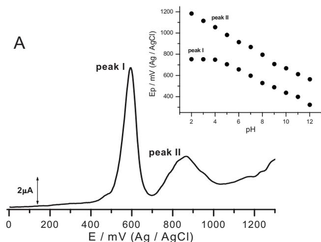
**Figure 6.** DP voltammogram of 1 mM 4-(3-indolyl)-DHP in 0.04 M Britton–Robinson buffer/ethanol (70/30) at pH 7. Inset:  $E_p$ /pH plot for 4-(3-indolyl)-DHP.
