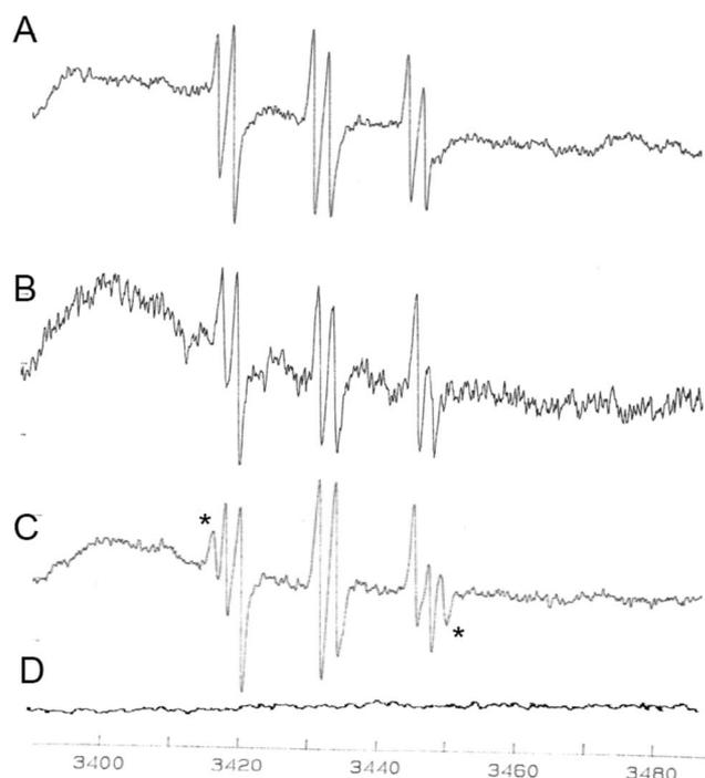
**Figure 5.** ESR spectra of 4-(3-indolyl)-DHP (A) and 4-(5-indolyl)-DHP (B) electrolyzed solutions at 1100 mV. (C) ESR spectrum of 4-(5-indolyl)-DHP electrolyzed at 1500 mV (\* New signals). (D) ESR spectrum of 100 mM PBN electrolyzed at +1500 mV in DMSO +0.1 M TBAPF6.
