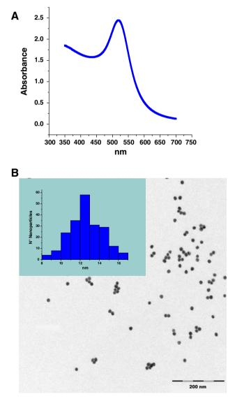
**Fig. 1.** Characterization of gold nanoparticles. GNPs were synthesized following the procedure described by Levy et al. [15]. (A) UV–Vis spectra of 5 nM GNPs and (B) transmission electron microscopic analysis of the particle morphology and size. The inset shows the distribution diameter of the GNPs obtained.
