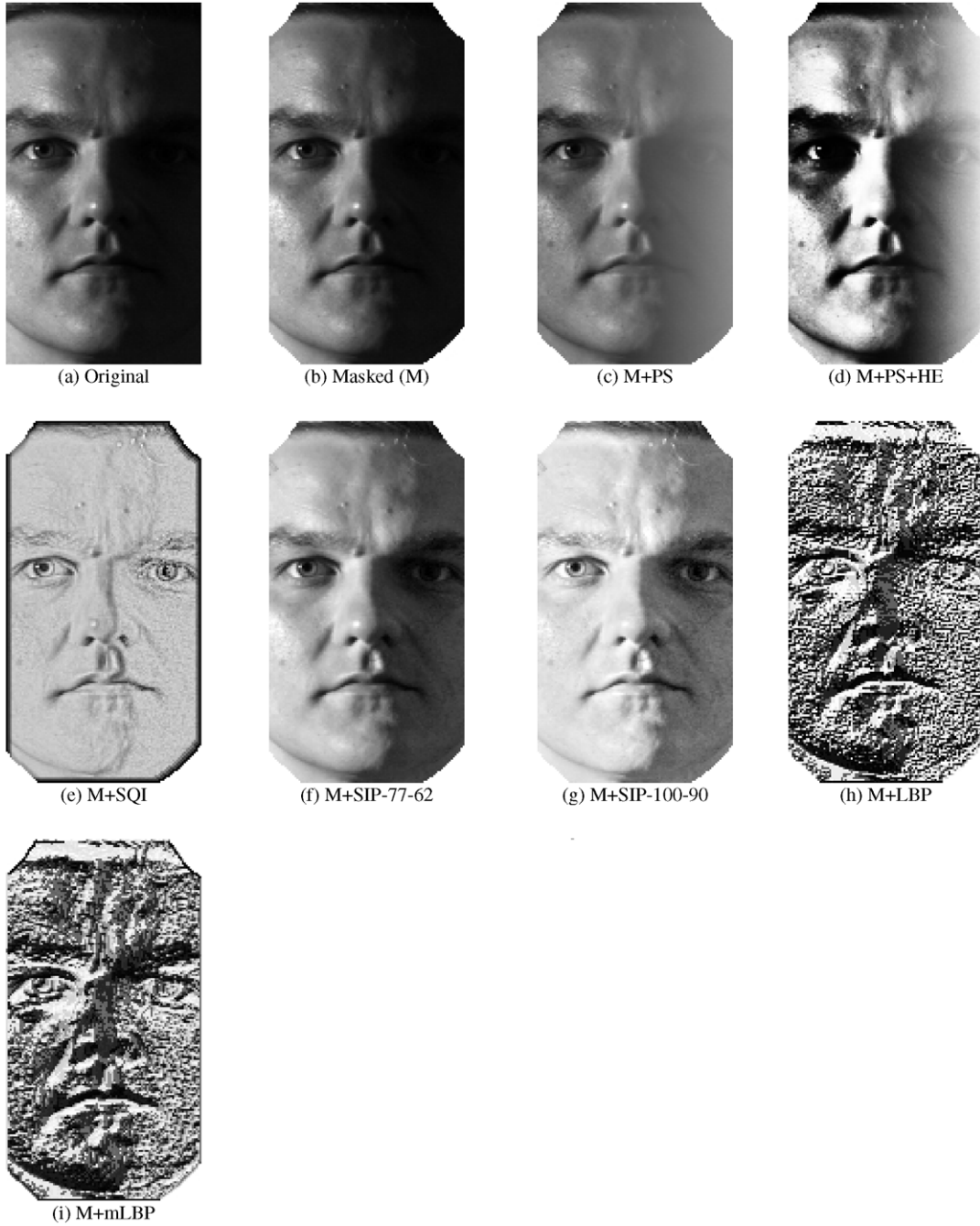
Fig. 1. Example image of an individual from the Yale B database (a). The image is pre-processed by masking the central part (b). Afterwards several illumination invariant algorithms are applied (c–i). PS: illumination plane subtraction; HE: histogram equalization; SQI: self-quotient image; SIP: Gross and Brajovic’ algorithm implemented by Shadow Illuminator Pro; LBP: local binary pattern; mLBP: modified LBP. See Section 3.2 for details.
