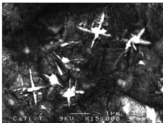
Figure 4. SEM micrograph of a \text{CaTiO}_3 film on titanium.
