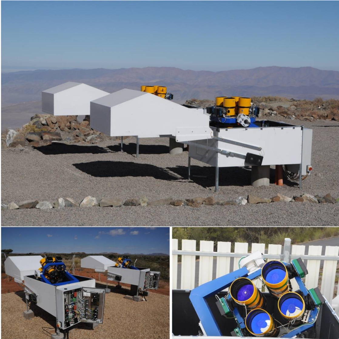
FIG. 4.— HS_4 units at Las Campanas Observatory, Chile ( top ), with the telescopes pointing towards the zenith. The HS_4 units at the HESS site in Namibia ( bottom left ), with telescopes stowed towards the south celestial pole. The electronic boxes are open showing the dome and telescope electronics described in § 2.1.5. A close-up view of an HS_4 unit at Siding Spring Observatory in Australia ( bottom right ), with part of the wind fence visible in the background. See the electronic edition of the PASP for a color version of this figure.
