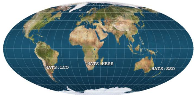
FIG. 5.—Geographical location of the HATSouth sites on a Mollweide projection. These sites provide near-optimal longitudinal separation, with \text{LCO} \rightarrow \text{SSO} = 141^\circ , \text{SSO} \rightarrow \text{HESS} = 133^\circ , and \text{HESS} \rightarrow \text{LCO} = 86^\circ . The three sites enable round-the-clock monitoring of selected southern stellar fields (image generated by xplanet ). See the electronic edition of the PASP for a color version of this figure.
