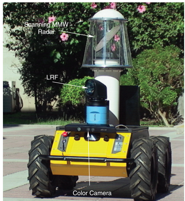
Figure 1. The Husky A200 with a camera, an LRF, and an MMW radar.
