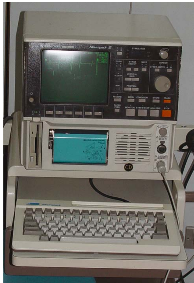
Fig. 1 Nihon-Kohden II machine (Evoked potential/Electromyographs, Nihon-Kohden Co., Japan), generating 2–50 mA per pulse of faradic continuous electric current (square wave pattern)
