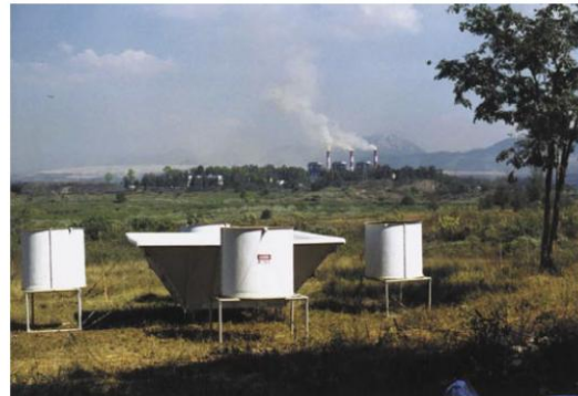
Vaisala LAP®-3000 with optional RASS for air quality monitoring.
