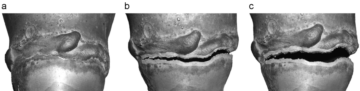
Fig. 13. Three levels of damage introduced to the car exhaust system.
