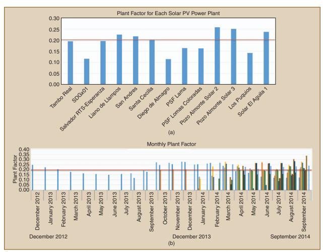
**figure 5.** (a) The plant factor of existing solar power plants and (b) the monthly plant factor, December 2012–September 2014 (source: CDEC-SIC).
