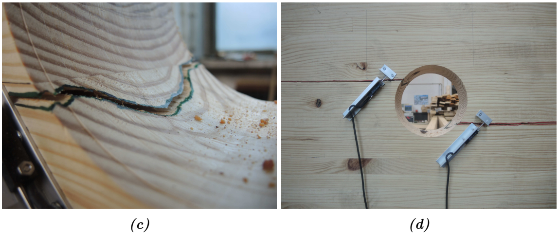
Figure A.4: Figures of the specimen S_3 (without reinforcements) after failure.
