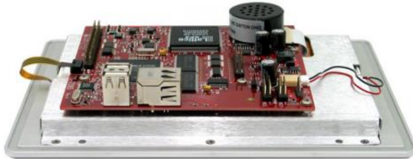
Figura 2-11: Single Board Controller (SBC) [3].
