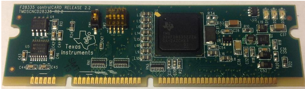
Figura 2-10: DSP TMS320F28335 Release 2.2.
