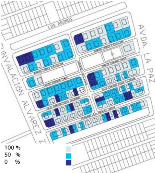
Figure 8: changes to housing permeability in Villa Las Araucarias housing development, La Serena.
