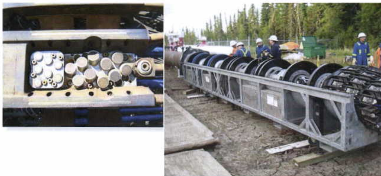
Figure 10: a. sensor plate, b. 40" tool prior to launching
