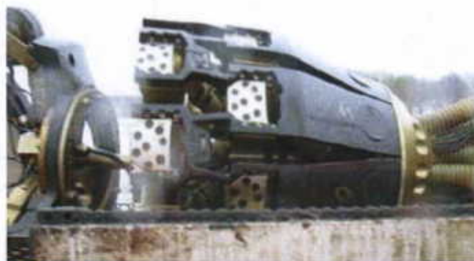
Figure 14: Modified sensor carrier; clean after run in high wax content line
