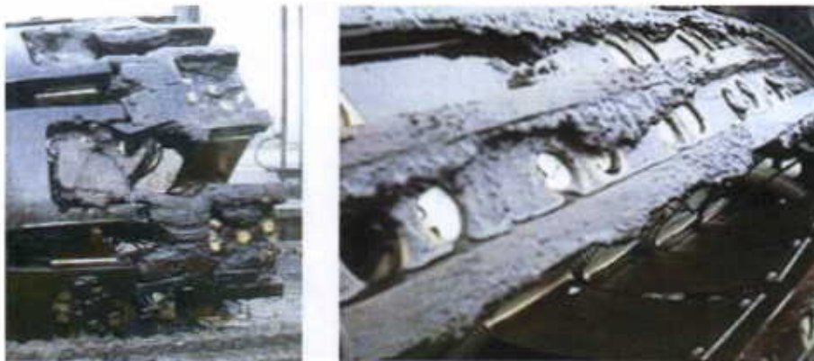
Figure 13: Wax built up on sensor carrier
