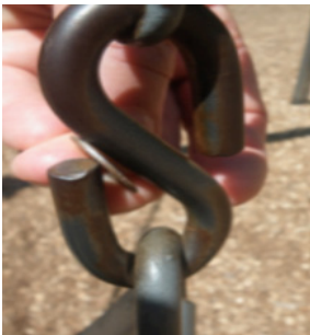
Figura Enredo Gancho s cerrado Fuente: Menke, Ron (2013) Safer Playgrounds. Facilities Solutions.
