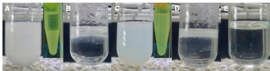
Figure 2. Mixtures of PEO 43 - b -PCL 14 (50 mg/mL), organic solvents, and water (10 wt %): (A) toluene, (B) chloroform, (C) cyclohexanone, (D) dichloromethane, and (E) acetone. Insets: corresponding samples after centrifugation.
