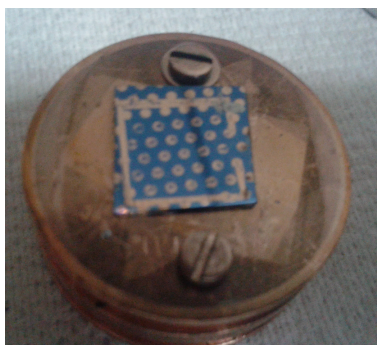
Figure 2.5: Sample with the point contacts used for the surface potential measurement
