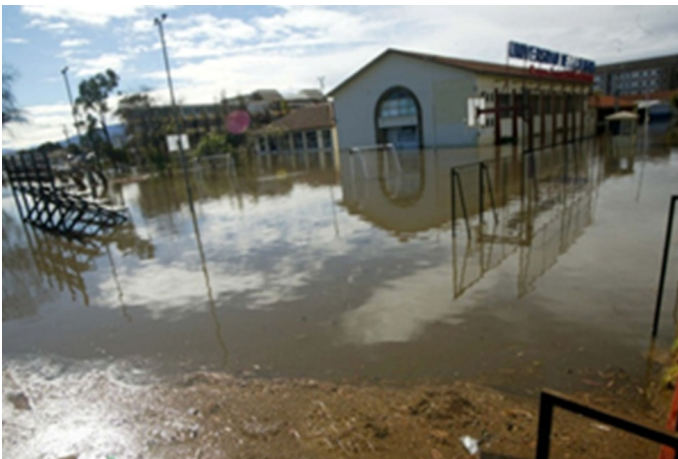
Fig. 14 Flooded areas at University of La Serena on the lower marine terrace after 70 mm/24 h rainfall in 2011. The flooding is a consequence of poor infiltration characteristics of the soil. Source: www.emol.cl
