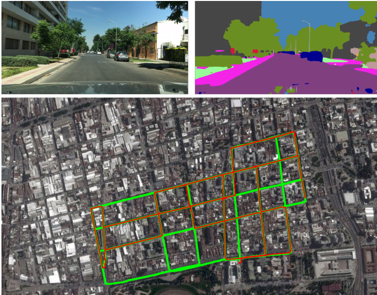
Fig. 4 Top: An example of the recorded database, the input image and the outcome of the segmentation algorithm [32]. Bottom: a satellite image showing the routes traveled in the dataset.
