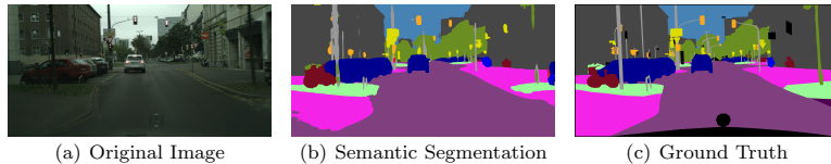
Fig. 2 Semantic Segmentation Example: (a) shows an image from the Cityscapes dataset[10], (b) shows the results of [32], and (c) is the ground truth of the dataset.
