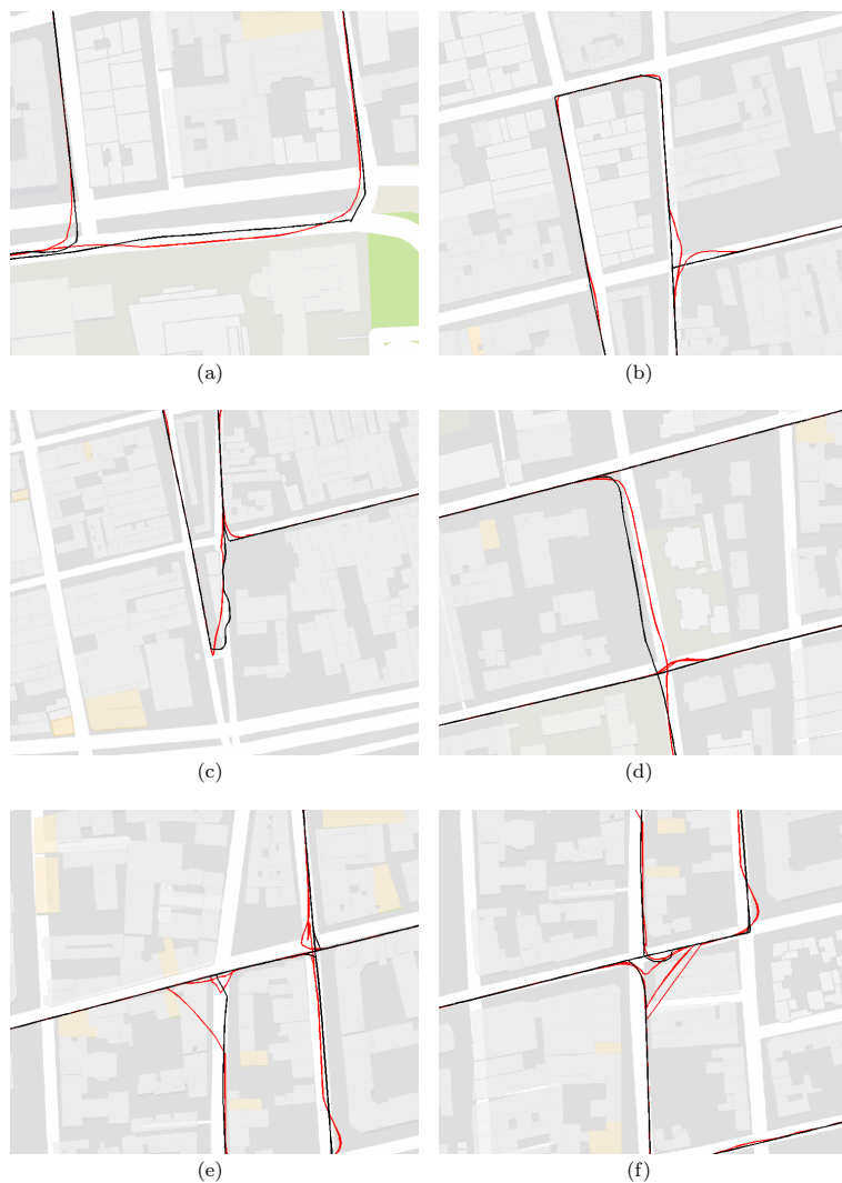
Fig. 8 Error examples of the proposed method. (a) displays an error related with driving on a different lane in the same road. (b) shows the effect of the particle dispersion in the pose estimation near an intersection. (c) and (d) show GPS related errors, as the ground truth poses are outside of the road in the map. And (e) and (f) show intersections where pose estimation goes wrong but is soon corrected.
