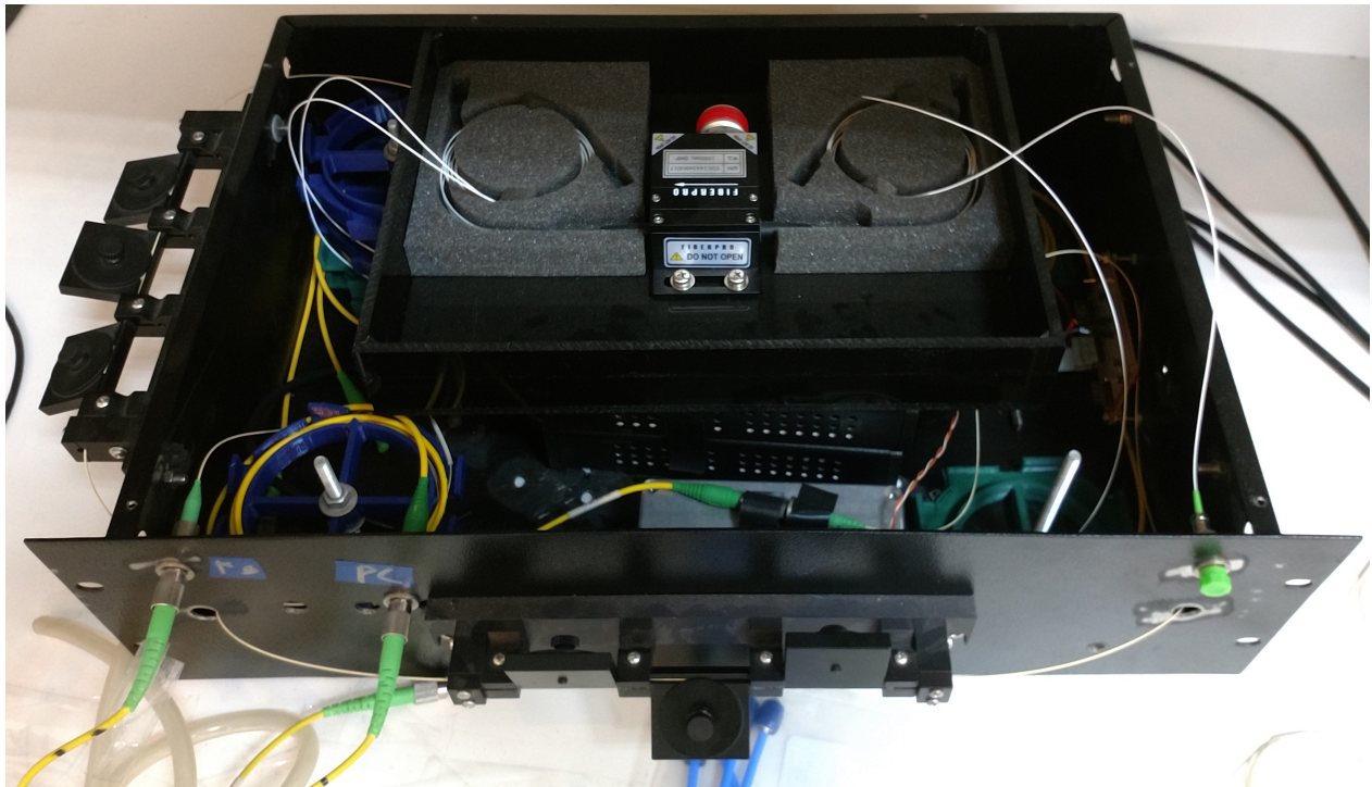
Figure 3.2: LO distribution box.
