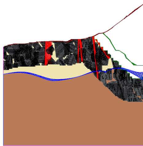
Figure 19. SM section view with deterministic joints in red and DFN in black
