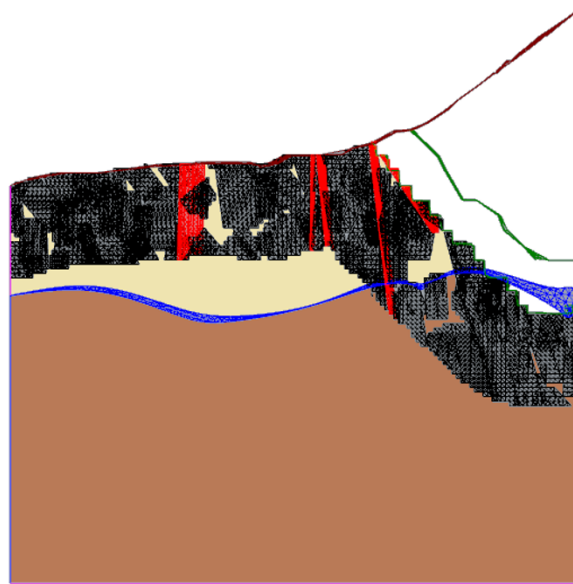
Figure 29. Model created with SM. Geometries DFN (black) and deterministic joints (red)
