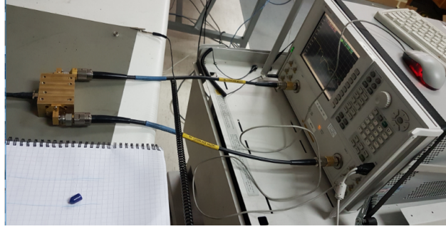
Figure 3.16: Photo of connection of VNA with final block.
