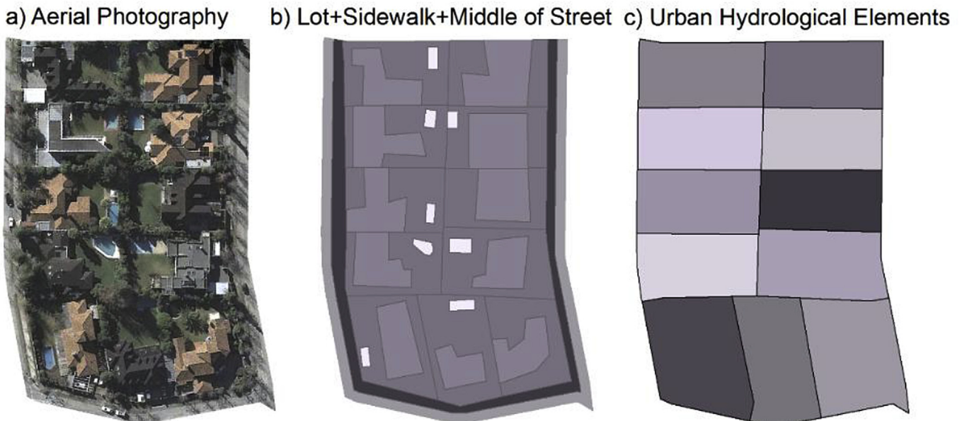
Fig. 4. Example of UHEs generation in Geo-PUMMA. (a) Aerial Photography; (b) Lot + Sidewalk + Middle of street in front of each lot, and (c) final UHEs map.
