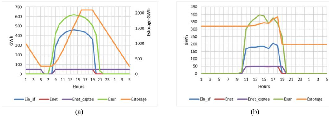
**FIGURE 3.** Production for base case: a) clear day, b) partial day. Ein\_sf: Energy in SF, Enet: Energy net without TES, Enet\_csptes: Energy net with TES, Esun: Energy from sun, Estorage: Energy storage.
