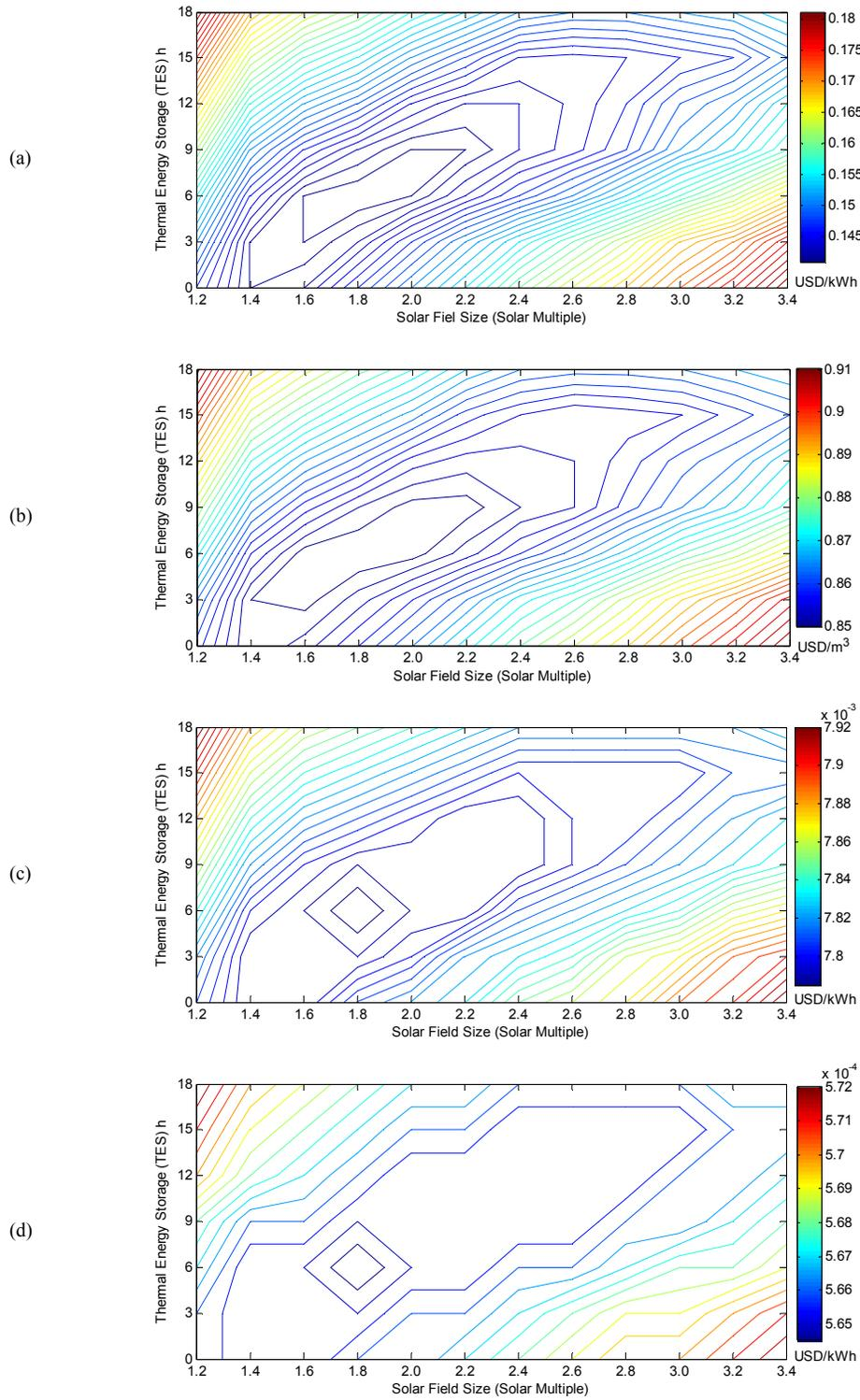
FIGURE 7. Levelized cost of a) electricity (LEC), b) water (LWC), c) cooling (LCC), d) heat (LHC).
