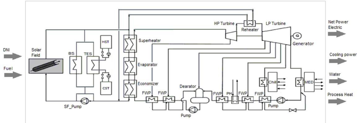
FIGURE 1. Polygeneration plant configuration. CSP/TES + MED + Chill + PH.
