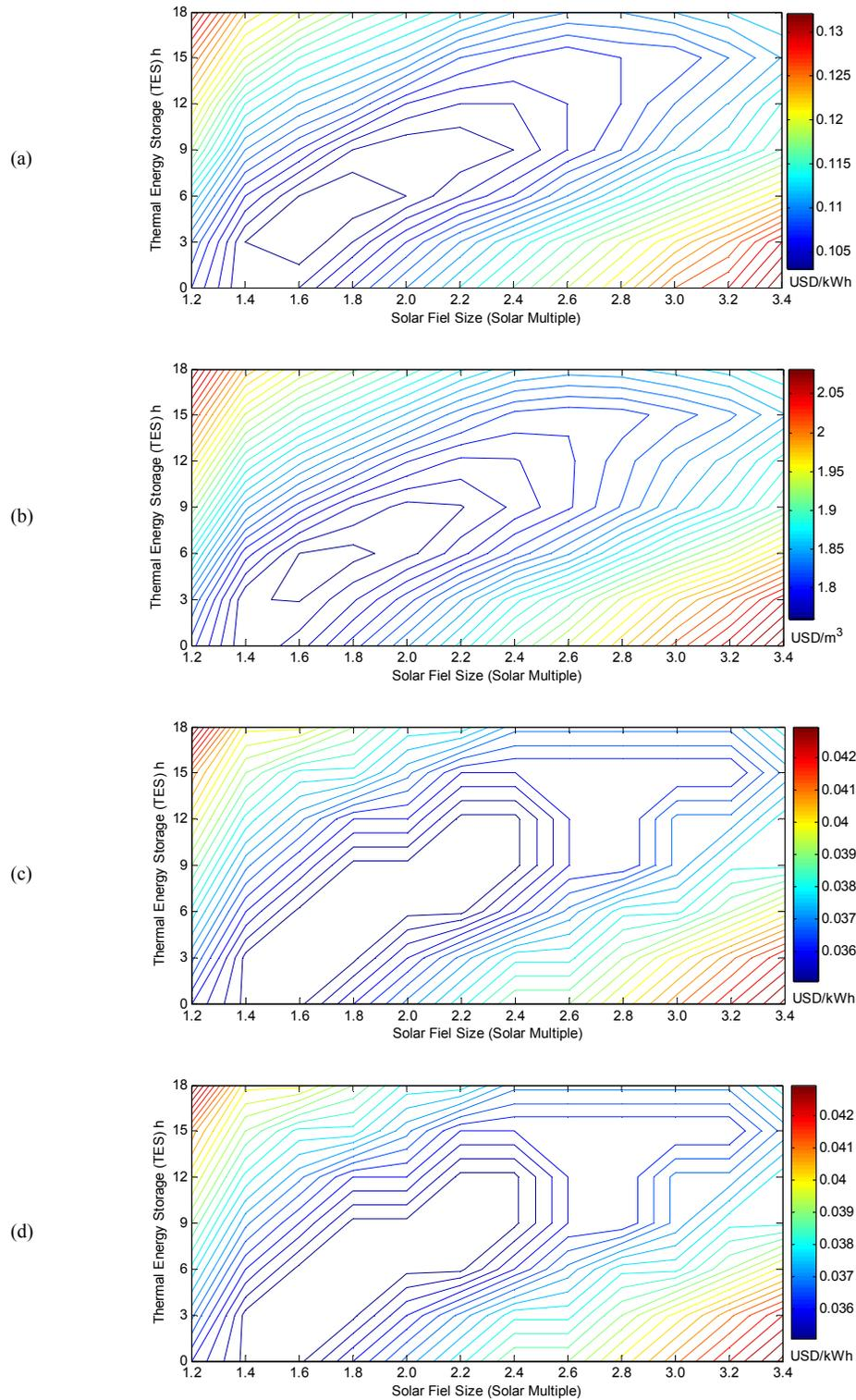
**FIGURE 6.** Exergy unit cost of a) electricity, b) water, c) cooling, d) heat.
