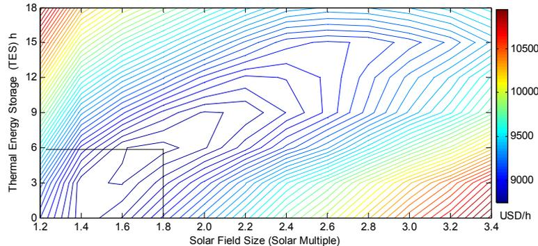
**FIGURE 5.** Total exergy cost rate of products USD/h in function of solar multiple (SM) and hours (h) of TES.
