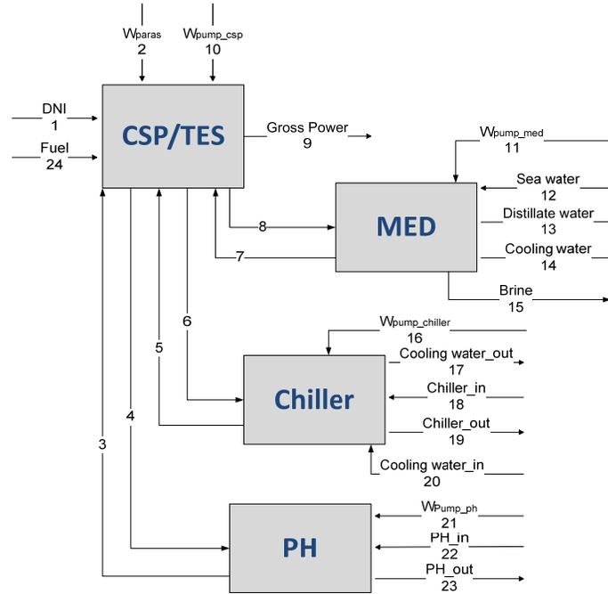
FIGURE 2. Aggregation level for exergoeconomic assessment in polygeneration plant.
