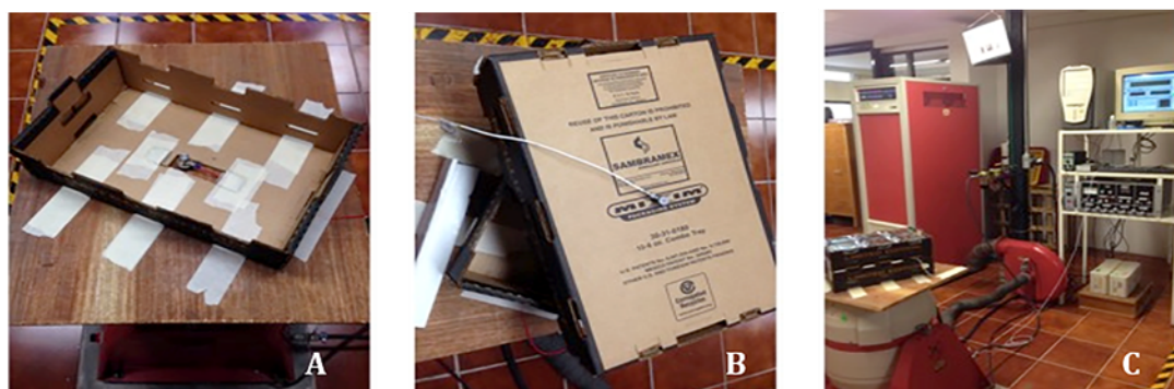
Figure 1. Experimental scheme to study the vibration profile. Accelerometer placed on the vibration table (A), accelerometer placed in the center of the bottom of the second box containing clamshells with blackberry 6 oz (B), an overview of all electro-hydraulic vibration system to simulate vibration in transit (C).
