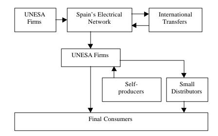
Figure 10.1. Simplified Operations of the Electricity System in Peninsular Spain
