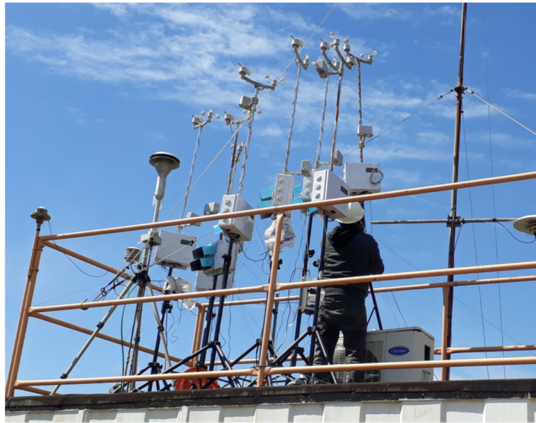
Fig. 3. Low-cost sensors on top of a pollution monitoring station located inside the Enap Oil Refinery during calibration procedure.
