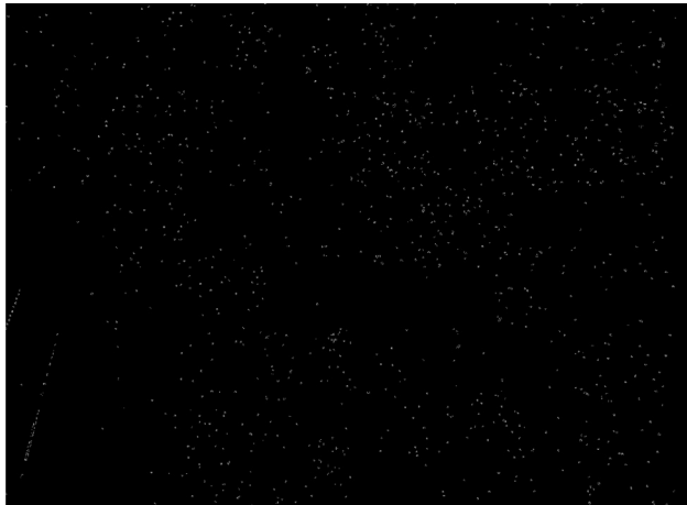
Fig. 8. Results of applying Canny Edge Detector without contrast stretching. Only the brighter stars were detected and airplane streaks, but does not detect any of the SO edges.
