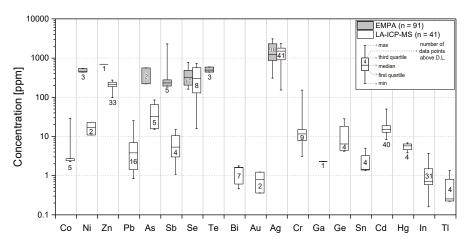
**Figure 3.** Boxplot of EMPA and LA-ICP-MS data for selected minor and trace elements in chalcopyrite from the Cerro Pabellón geothermal system. Analyses are plotted in parts per million (ppm) on a vertical logarithmic scale. The maximum, median, and minimum concentrations are indicated, as well as the number of analyses above the detection limit for each element (displayed inside or below the boxes). Analyses with "spiky profiles" in Table S2, attributed to inclusions, were not plotted.
