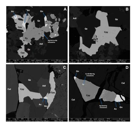
**Figure 2.** (**A**–**D**) show back-scattered electron (BSE) images of chalcopyrite from the Cerro Pabellón geothermal system. Chalcopyrite is euhedral to subhedral and is mostly free of mineral inclusions, although some grains show Ag-bearing micro-inclusions (e.g., (**D**)) and larger inclusions of Cu–S–Sb–Ag-bearing minerals (e.g., (**A**) and (**D**)). Abbreviations: chalcopyrite (Cpy), pyrite (Py), acanthite (Ac), galena (Gn), adularia (Adl), calcite (Cal), quartz (Qz).
