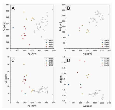
**Figure 5.** Bivariate plots showing Cu–Ag (**A**), Zn–Ag (**B**), Cd–Ag (**C**), and In–Ag (**D**) trends for chalcopyrite from the Cerro Pabellón geothermal system. Samples BA-20 and BA-48 are the shallowest (494 m) and the deepest (549 m), respectively, and show distinct variations in trace element concentrations. All plotted data correspond to inclusion-free LA-ICP-MS analyses (see Table S2).
