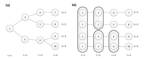
**Figure 1.** A scenario tree consisting of four scenarios and four stages (time periods) and 10 nodes (1a) is shown. The scenarios are also shown in a disaggregated form (1b); the non-anticipativity constraints (information sets Nt) are reflected by the balloons grouping the nodes. For example, in period two (t = 2) node two shares scenarios one and two and therefore the decisions for this node (harvest or not harvest the stand) for scenarios one and two must be the same.
