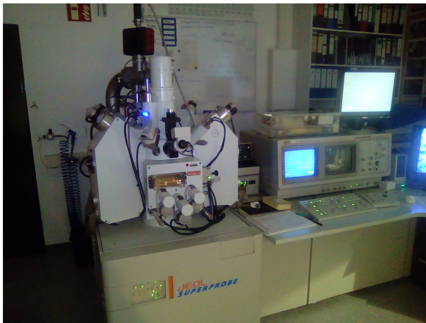
Figure 4.6: Electron Micro Probe (EMPA) in Geoscience center (GZM), George-August University of Göttingen. The picture shows the vacuum chamber where we introduced holders and thin sections for analysis.
