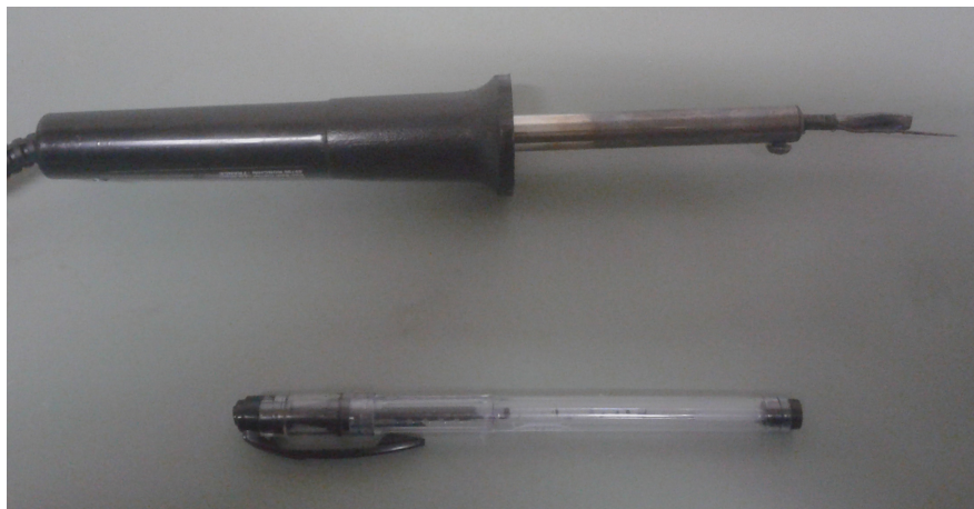
Figure 4.4: High-temperature needle used to liberate minerals from Epoxy mounts. The needle is plugged into the electrical socket and works by resistance. By increasing the current, the temperature increases and allows the needle to locally melt the necessary epoxy to “free” the crystals.
