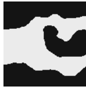
Figure 1.3: Categorical permeability channel. Example of a 2-D representation of a categorical channelized permeability field.
