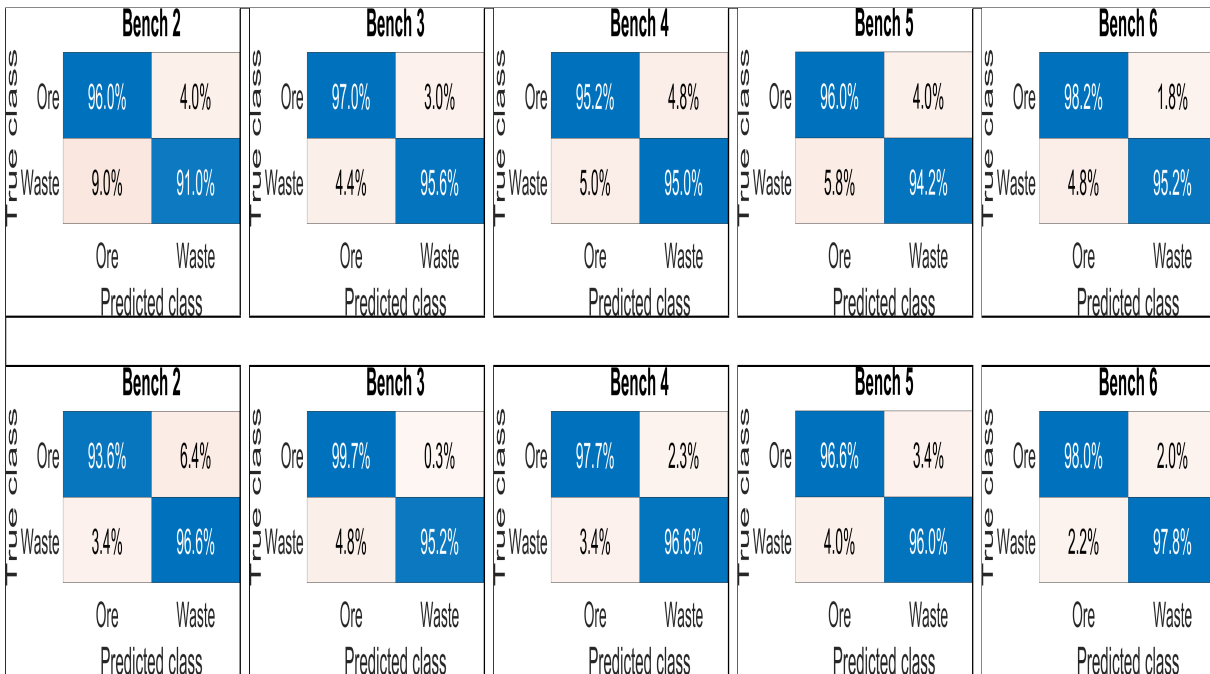
Figure B.18: Confusion Matrix for Case Study 3. From left to right: Benches 2-6. Top: Structured sampling. Down: Adaptive sampling using Cut-Off grade 0.115%.
