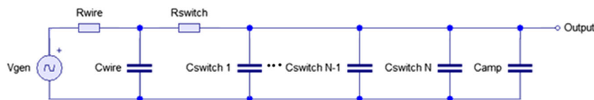
Figure 3. Schematic of parasitic elements for one channel: R_{\text{wire}} , wire resistance; C_{\text{wire}} , wire capacitance; C_{\text{switch}} , switch capacitance; and, C_{\text{amp}} , amplifier resistance.
