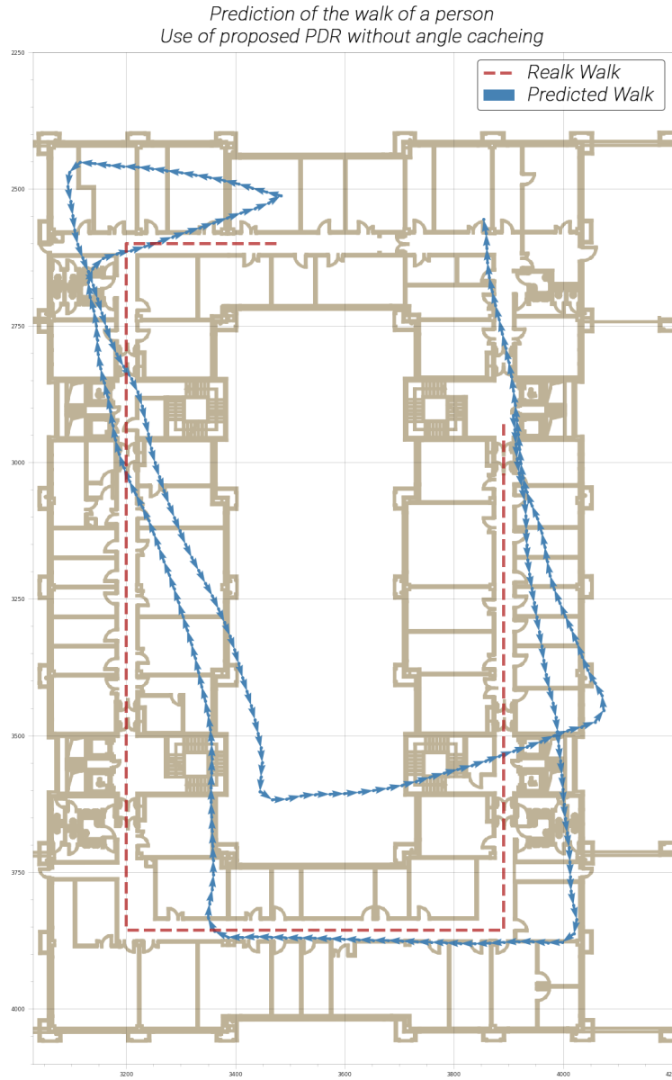
Figure 7.1: PDR system result for Route 1 in CNR, Pisa. No orientation cache.
