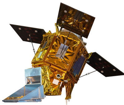
Figure 3.9: Example of Satellite taking measurements from the Earth. In this case is the Sentinel-5 Precursor satellite, which has the TROPOMI radiometer. AOD products are developed from the data obtained by this satellite (taken from Wikimedia Commons under CC BY 3.0 license).
