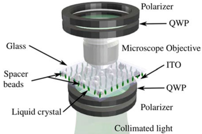
Fig. 1 Sketch of the experimental setup of a nematic liquid crystal layer with negative dielectric constant anisotropy and homeotropic anchoring under the influence of a voltage. The essential parts of the setup are emphasized. Crossed polarizers, either linear or circular are used to analyze the texture of the liquid crystal
