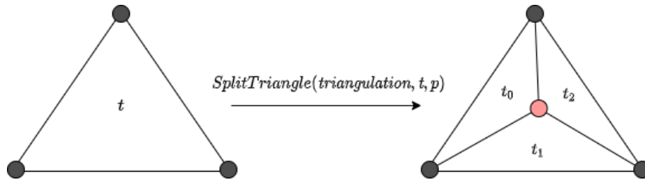
Figure 2.4: Graphic representation of the SplitTriangle function.
