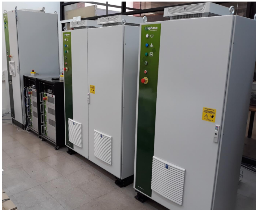
Figure 5.9: Experimental system based on five Triphase power converters, nominal powers 5-30kW (each one). They are configured to emulate the topology of Fig. 5.8.
