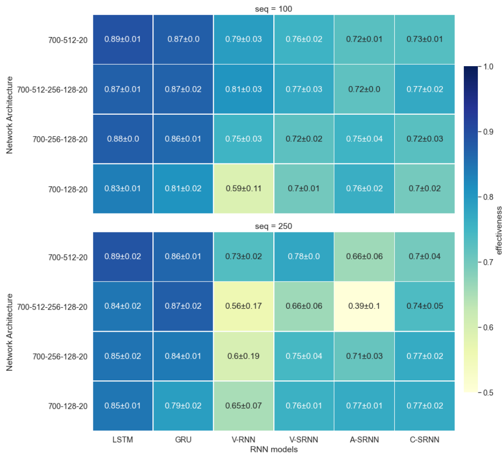
Figure 4.5: Mean accuracy and standard deviation of traditional RNNs and SRNN models for the SHD dataset.
