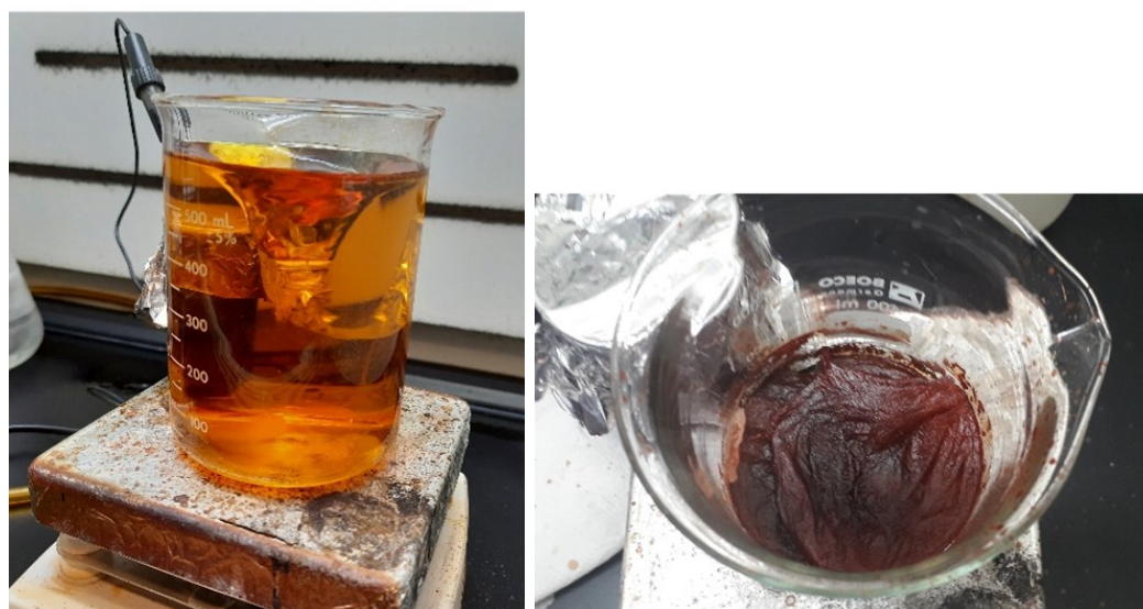
Figure 3.1: (a) Dissolving metal nitrites in distilled water and (b) Dried gel
