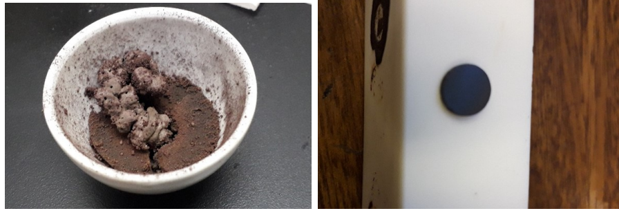
Figure 3.2: (a) Drying in oven, (b) Calcination in heat treatment furnace, (c) Calcined powder and (d) Disc shaped Sintered sample
